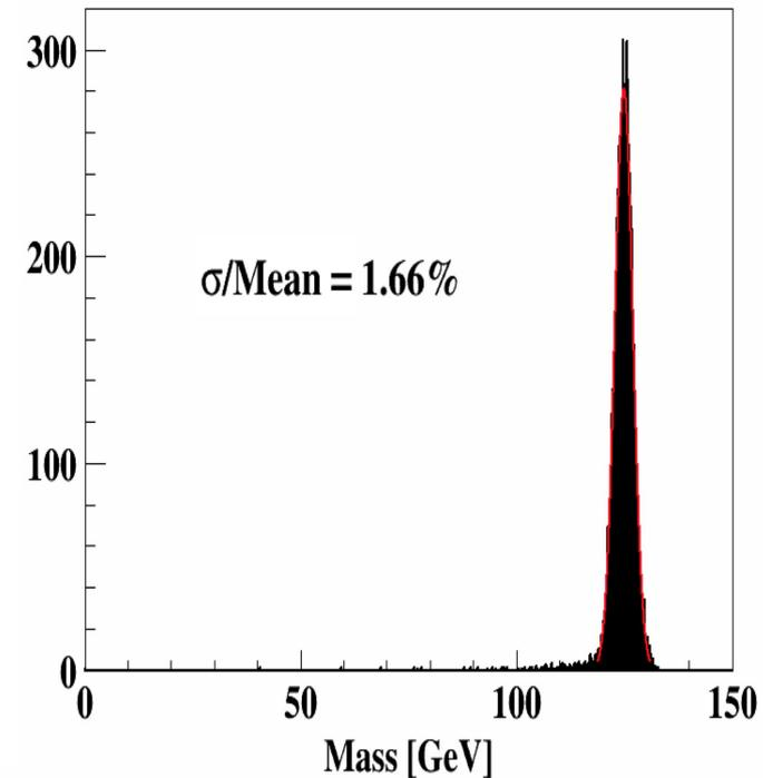
H  $\rightarrow$   $\gamma\gamma$  at CEPC-v4/Simplified geometry
