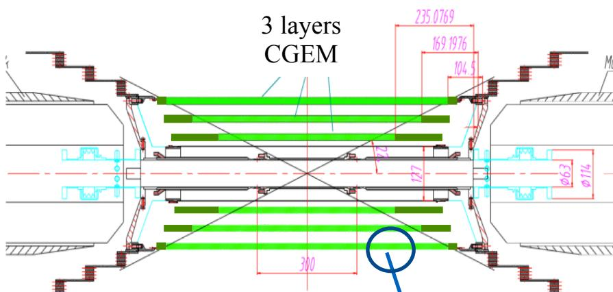
Each layer composed by a triple cylindrical GEM
