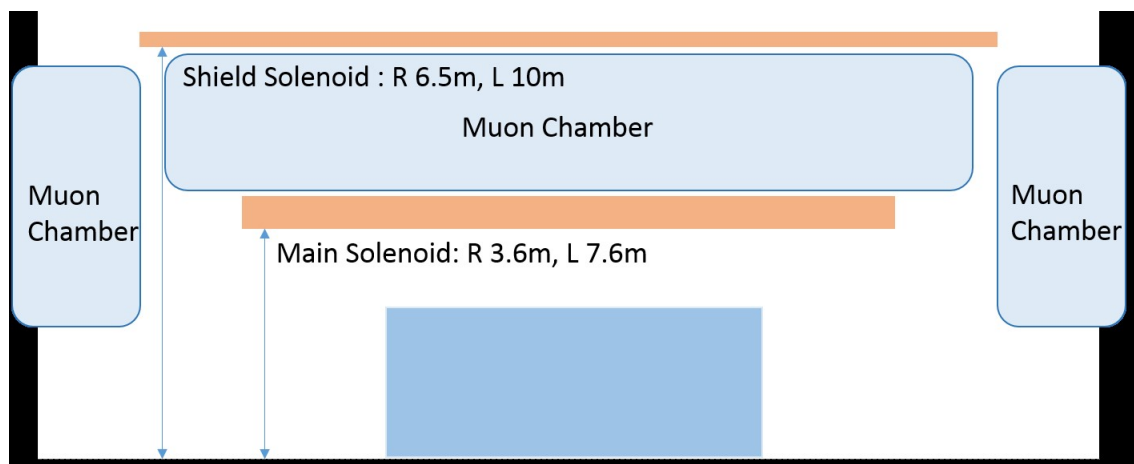
Figure 6.49: Sketch figure for the half cross section of the active shielding magnet, with the available areas for muon chambers
