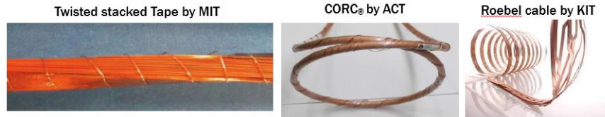
Figure 6.26: different YBCO cables
