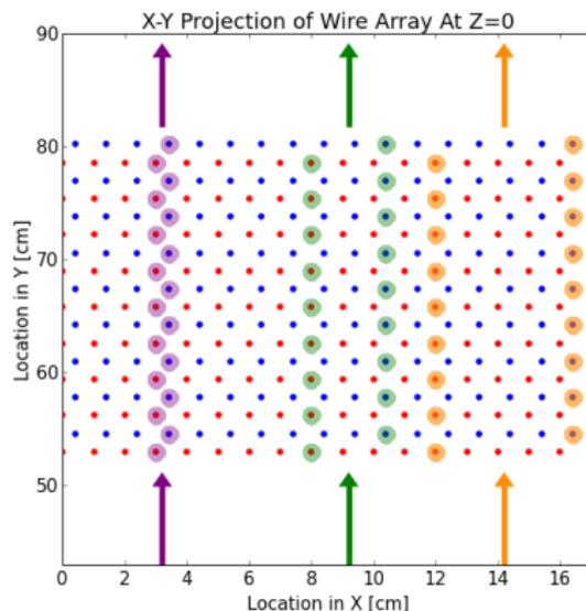
Figure: A projection at  $Z = 0$  of a wire array with alternating stereo angles from along the beamline.
