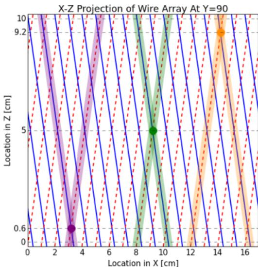
Figure: A projection of a wire array with alternating stereo angles from above.
