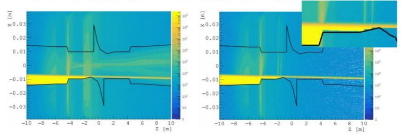
Number of photons per bunch hitting the central beam pipe dropping from 40, 000 to 80; power deposition reduced considerably
