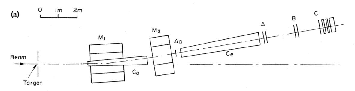
M1, M2: magnet, decouple the angle and the momentum of the particle
