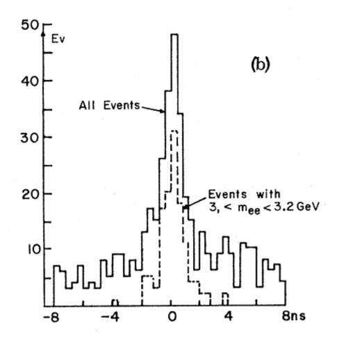
The time-of-flight spectrum between the e<sup>+</sup> and e<sup>-</sup> arms in the mass region 2.5<m<3.5GeV, a clear peak of 1.5-nsec width is observed
