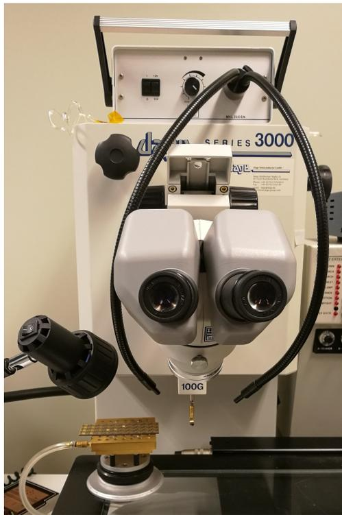
Figure 3.12: Photograph of the pull test machine *Dage Series 3000*. An extra light source is positioned on top of the pull test machine. The installed hook is a special hook which is only used for calibrations.
