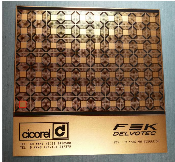
Figure 3.13: Photograph of the wire bond test material by *Cicorel*. The structure highlighted with red color indicates the regions used for test programs.
