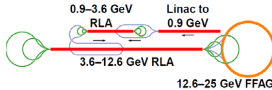
Figure 7. Low-energy acceleration system suitable for neutrino factory or muon collider.
