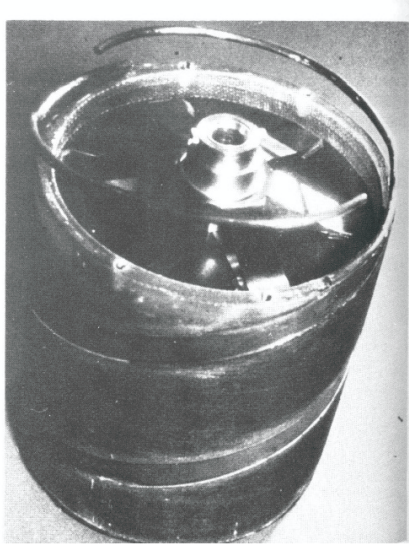
Figure 68. Vapor-cooled current lead on a cryostat turret (500 A, spiral wound leads, total length 150 mm between 300 and 4 K). Reproduced with permission from Scurlock (1988). Copyright 1988 Elsevier.
