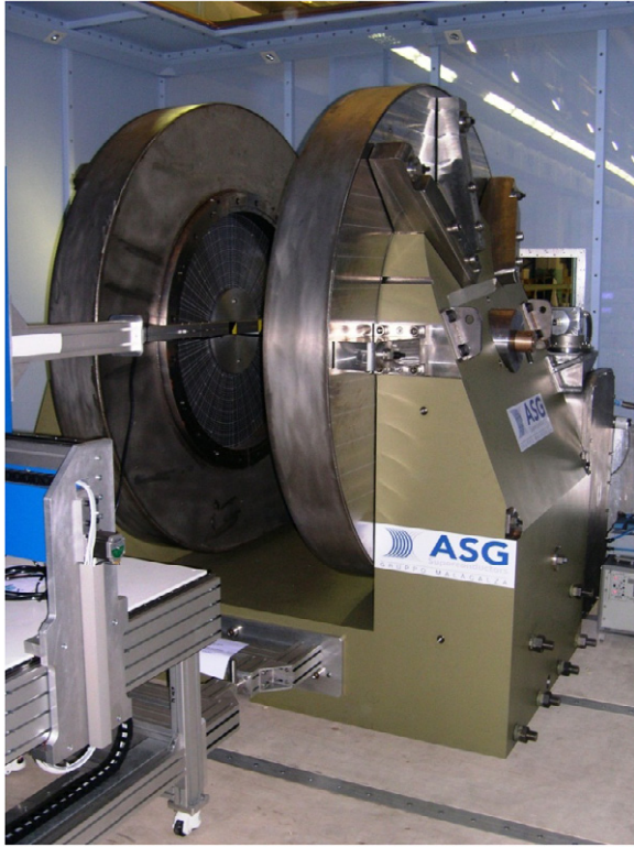
Figure 23. 0.5 T MgB 2 magnet, made by ASG Superconductor for Paramed OpenSky MRI scanner. Reproduced with permission from Modica et al (2007). Copyright 2007 IEEE.
