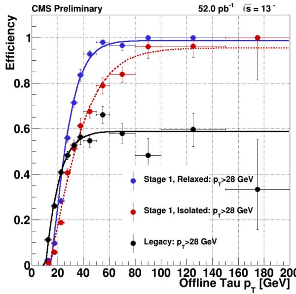
Run 2 major upgrade of the L1 trigger system increases the  $\tau_h$  collection efficiency.
