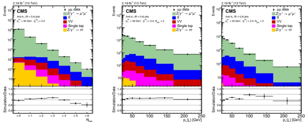
Data to simulation comparison of the exclusive jet multiplicity (left), and the  $p_T$  of second leading jet (middle) and third leading jet (right).
