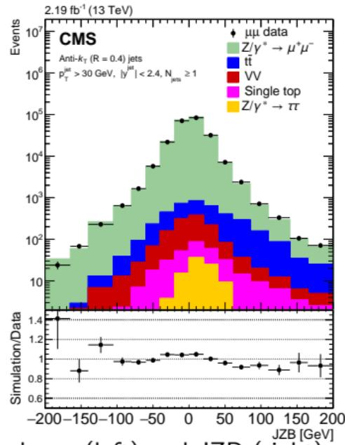
Data to simulation comparison of the  $p_T$  balance (left) and JZB (right) with  $N_{jets} \geq 1$ .
