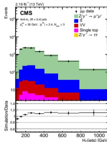
Data to simulation comparison of  $H_T$  of the jets for inclusive jet multiplicities of 1 (left), 2 (middle) and 3 (right) obtained for the  $\mu\mu$  sample.
