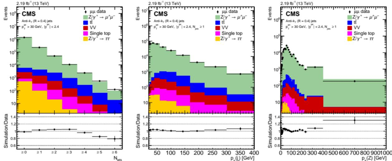
Data to simulation comparison of the inclusive jet multiplicity (left), the  $p_T$  of first leading jet (middle), and  $Z$   $p_T$  with  $N_{\text{jets}} \geq 1$  (right).
