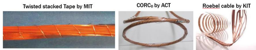
Figure 6.26: different YBCO cables
