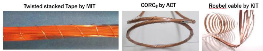
Figure 6.26: different YBCO cables
