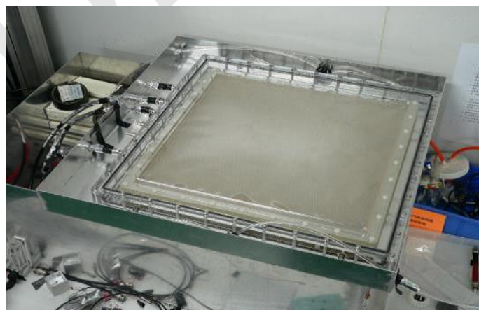
Figure 5.27: A double THGEM was produced with a size of 40 \times 40 \text{ cm}^2 .
