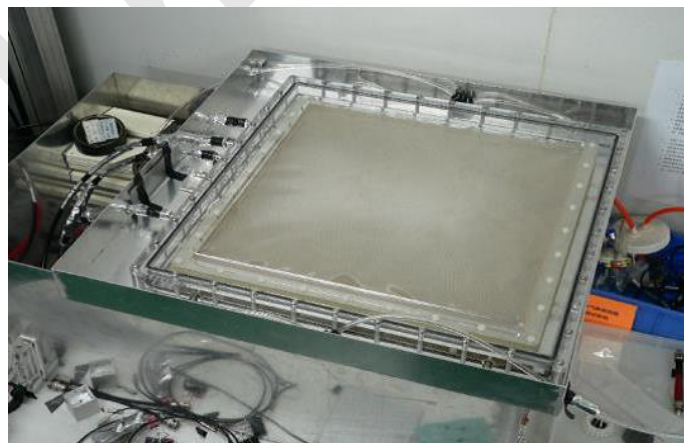
Figure 5.31: The maximum size of THGEM produced in domestic currently ( 40 \times 40 \text{ cm}^2 ).
