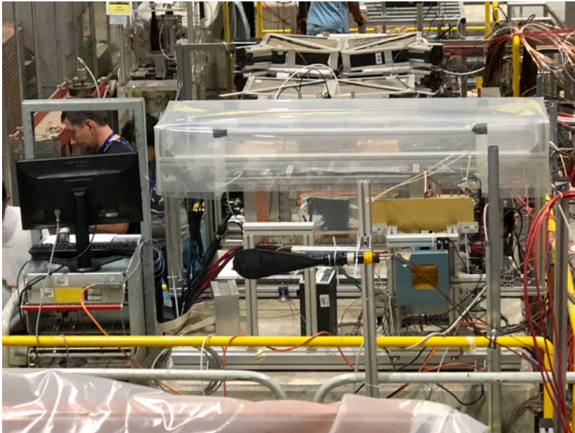
Beam test at CERN of a full IDEA slice: drift chamber, pre-shower, D.R. calo. \mu -counter.
