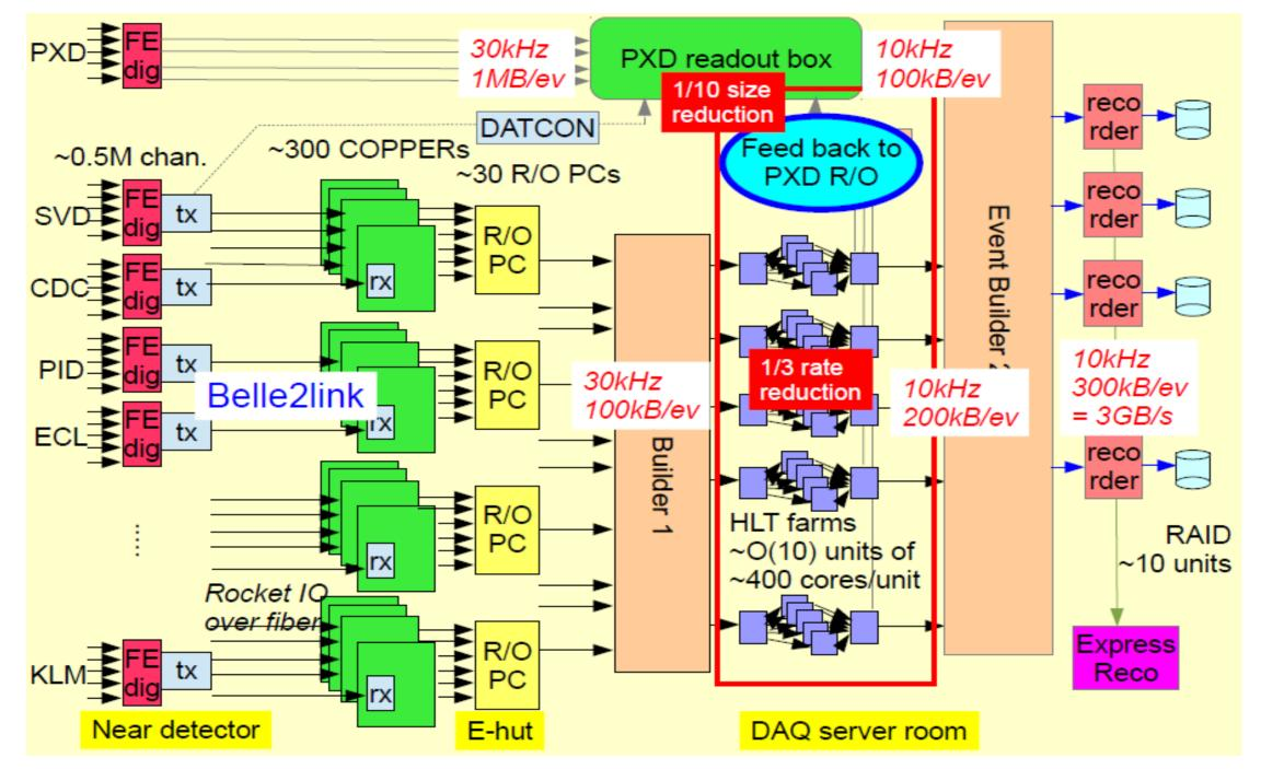
L1 trigger = 30 kHz Software Trigger = 10kHz
