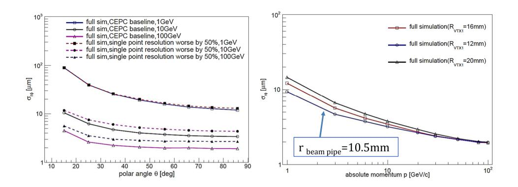
Sensitivity to single-point resolution and innermost radius with full simulation
