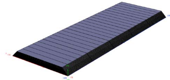
Figure 5.7: Schematic of the structure of one ECAL staff. Each staff is made up of 5 trapezoidal modules, and each module contains up to 5 columns.
