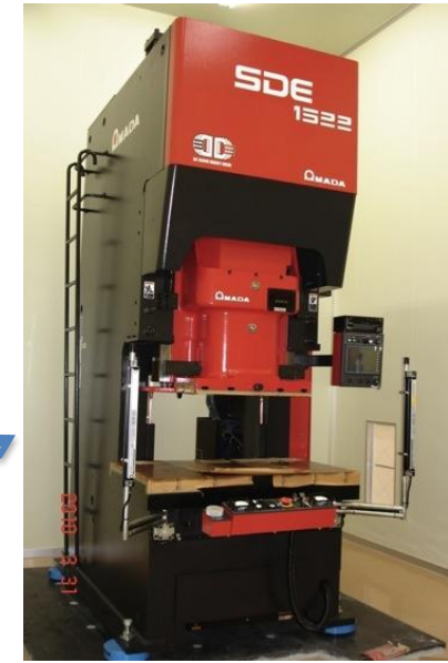
Servo press machine (AMADA, Japan) Max. applying force:1500 kN
