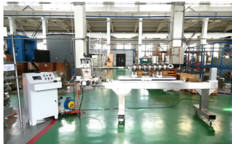
IHEP inner surface repairment equipment: 1.3GHz 9cell; 650MHz 5cell; 500MHz single cell
