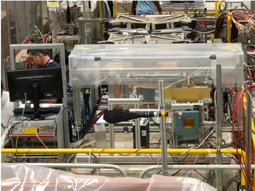
Beam test at CERN of a full IDEA slice: drift chamber, pre-shower, D.R. calo. μ-counter.
