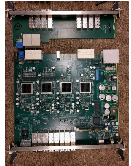
2 processing FPGAs + 2 fabric FPGAs
