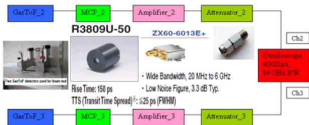
beam test detectors and DAQ
