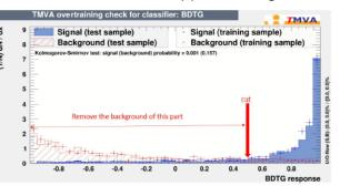
BDTG is chosen as the algorithm which would optimize the event selection and determine a BDT cut according to the maximum significance.
