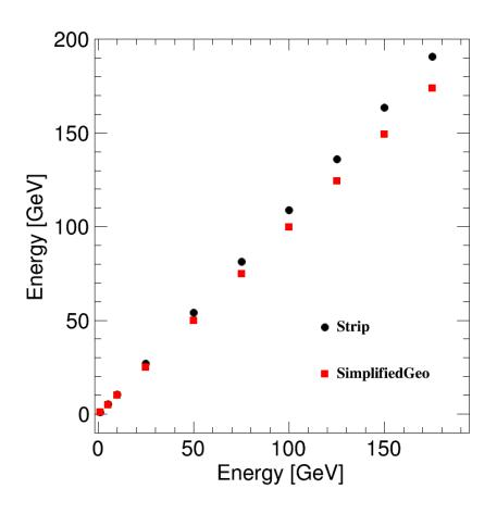
Some hits will be lost, when there is no energy deposition at the 18 cells for weight calculation
