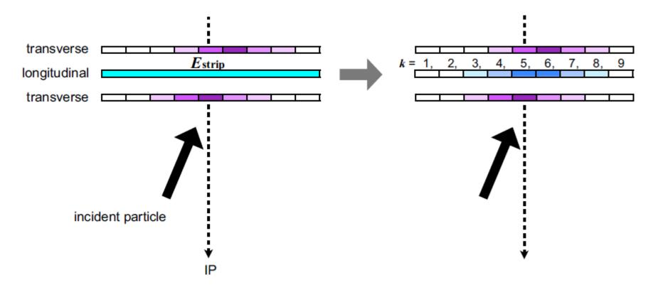
5\*45mm Cell -> 5\*5mm Cell Energies of Neighbor Layer Strips (2\*9) are used to calculate the splitting weights
