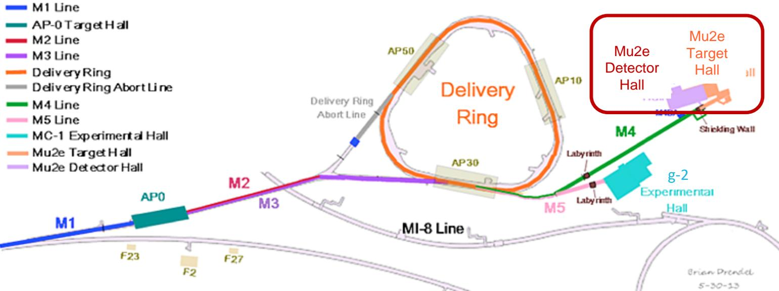
Beam into the M4 beamline from the Recycler + Delivery Ring will already have a between pulse extinction of  $10^{-4}$  or better
