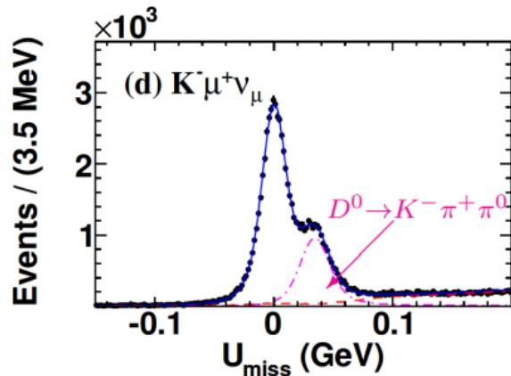
Hard for low momentum muon to hit the muon identifier, which leads to high background from pion misidentification.
