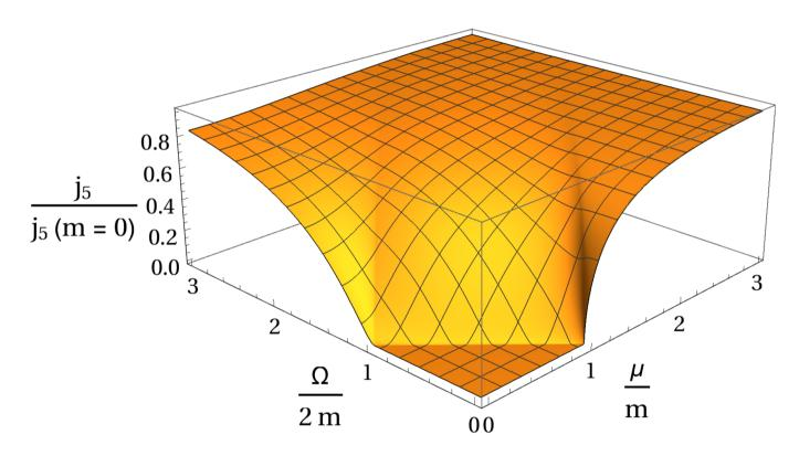
Axial current at  $\ T=0$  is zero in the region  $\ \Omega < 2(m-|\mu|)$  .
