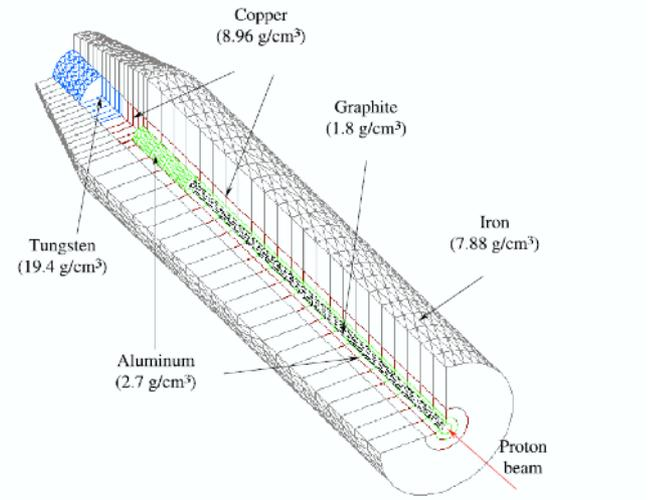
A perspective view of the FLUKA geometrical representation of the TED beam-dump.
