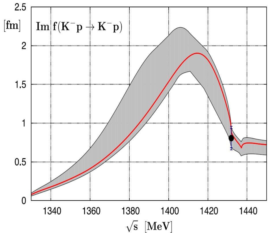
Real part and imaginary part of the  $K^- p \rightarrow K^- p$  forward scattering amplitude extrapolated to the subthreshold region, deduced from the SIDDHARTA kaonic hydrogen measurement.
