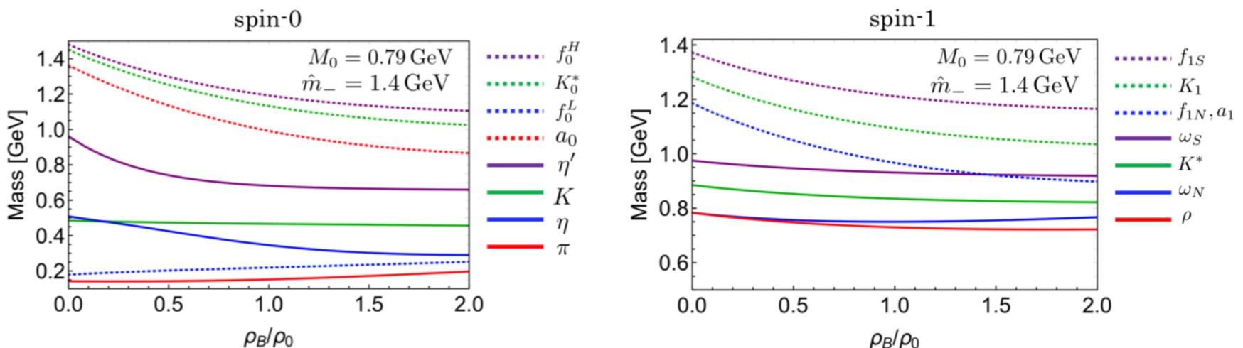
FIG. 6. (color online) The density dependence of spin-0 (left) and spin-1 (right) meson masses with  $\hat{m}_- = 1.4$  MeV,  $M_0 = 0.79$  GeV, and  $k_1 = k_2 = 0$ .
