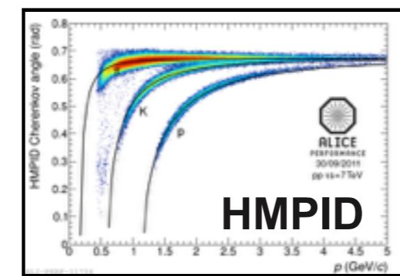
HMPID  $\sigma_{\text{Cherenkov Angle}} \sim 3 \text{ mrad}$
