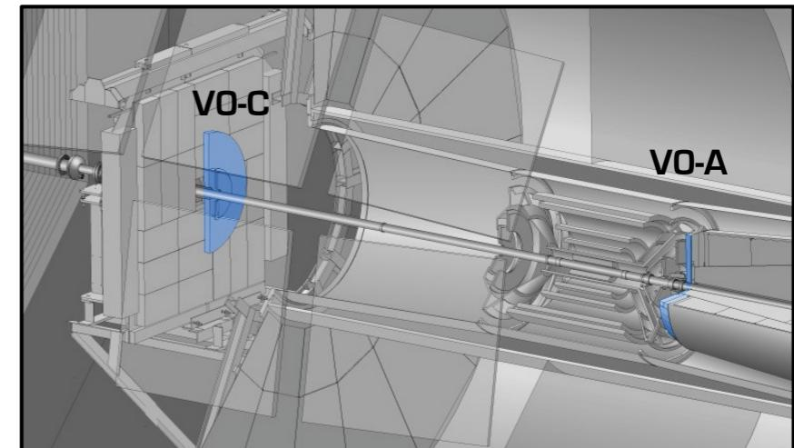
The VO detector is composed of a pair of forward scintillator hodoscopes placed at  $2.8 < \eta < 5.1$  (VO-A) and  $-3.7 < \eta < -1.7$  (VO-C)
