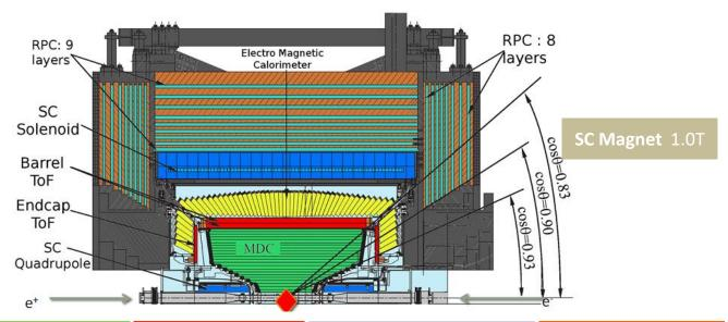
Main Drift Chamber Small cell, 43 layer  $\sigma_{xy}$ =130  $\mu$ m, dE/dx~6%  $\sigma_{n}/p$  = 0.5% at 1 GeV
