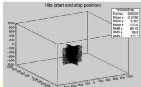
Distribution of  $e^-$  hits in 8 silicon radial detector vanes (after the decay of the muon in the stopping target) (in gray, → ,
