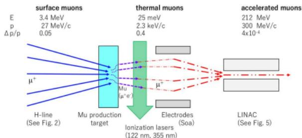
A new method to inject the muon beam !
