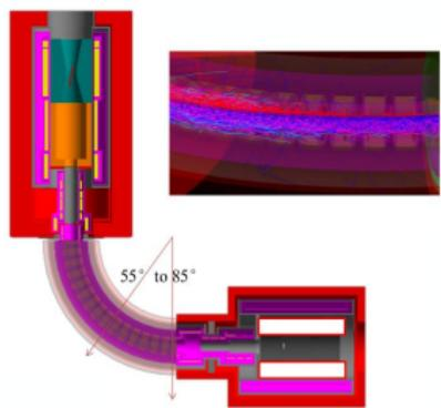
Figure 8.5: Schematic layout of muon beam collimators placed inside the muon transport solenoid from 55° to the end, and event displays (top right) with the collimators in place in the muon transport solenoids. Tracks in blue are  $p^-$ , those in red are  $p^+$ .
