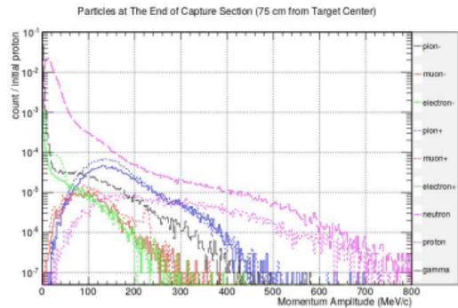
Figure 8.3: Momentum distribution of various beam particles at the end of the pion capture solenoid section, moving to the muon transport section. For the hadron production, GEANT\_QGSP\_BERT was used.
