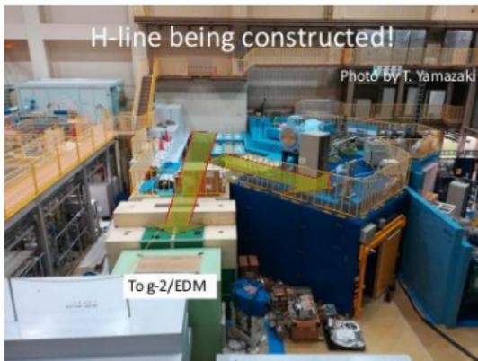
A 3 GeV primary proton beam with 1 MW beam power from the Rapid Cycle Synchrotron hits a 2 cm thick graphite target to provide pulsed muon beams. The experiment uses a surface muon beam. Surface muons are nearly 100 % polarized positive muons from pions stopped at and near the target surface. The H-line extracts muon beams.
