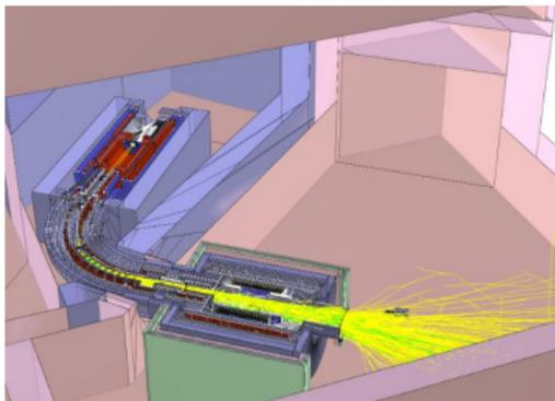
Phase-I layout of the COMET experiment, showing the first 90° bend of the muon transport beam line. The detector will be placed at the end of the muon transport section. (under construction )
