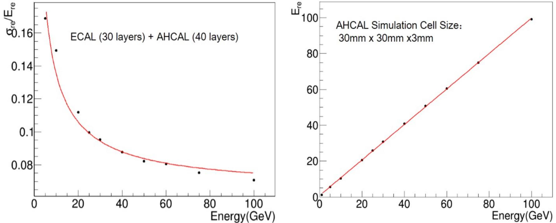
**Figure 5.32:** The left plot is the energy resolution from the SiW-ECAL and AHCAL for pions. The right plot is the corresponding results of reconstruction energy linearity. The energy resolution is 11% and 8% for energy at 20 GeV and 80 GeV, respectively.
