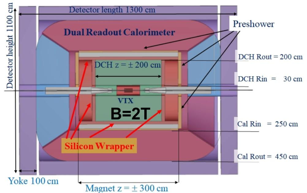
*Calorimeter outside the coil*
