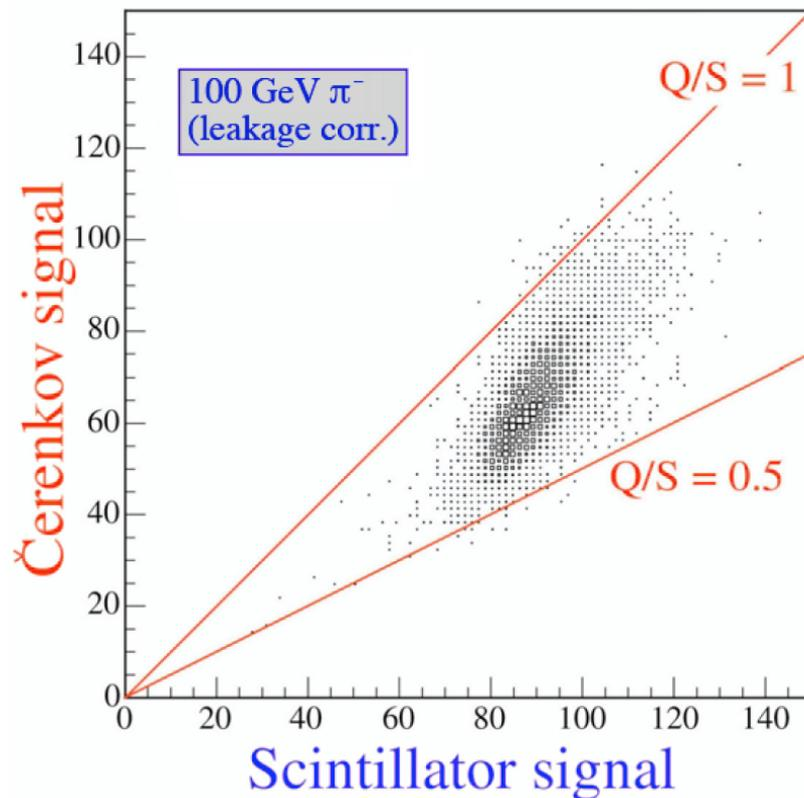
Reconstruct  $f_{EM}$  on an event basis  $\rightarrow$  Alternating quartz and scintillating fibers in metal matrix.
