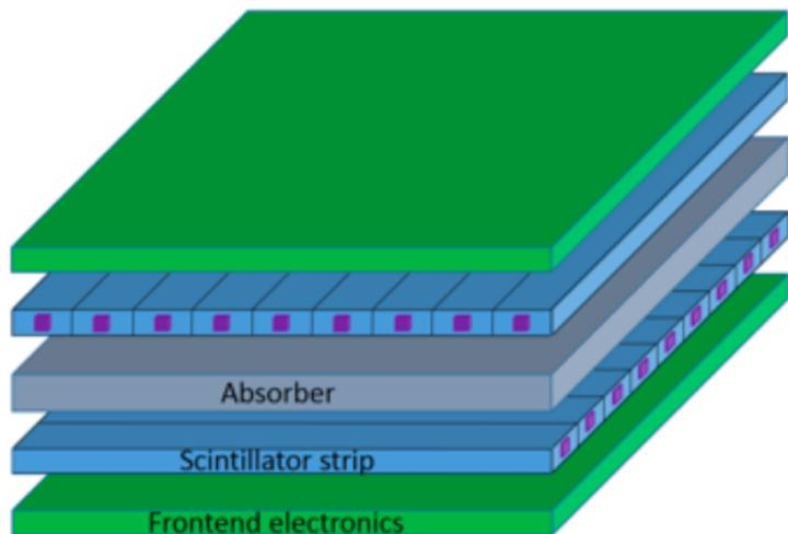
“Crossing” configuration of strips to get a high effective granularity
