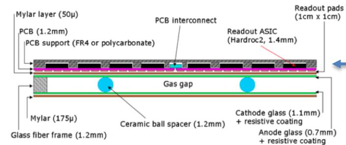
Embedded readout electronics
