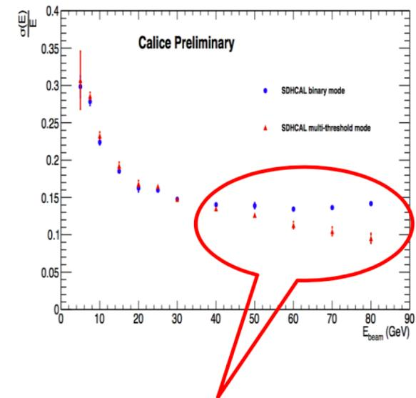
**SDHCAL with 3-threshold results in better energy resolution than binary mode for  $E_{\text{beam}} > 40$  GeV**
