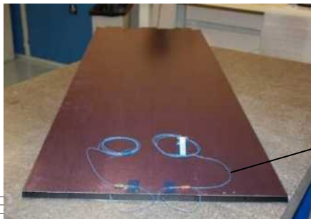
Optical fiber equipped with BG sensors
