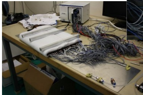
Active cooling set up test with water at room temperature
