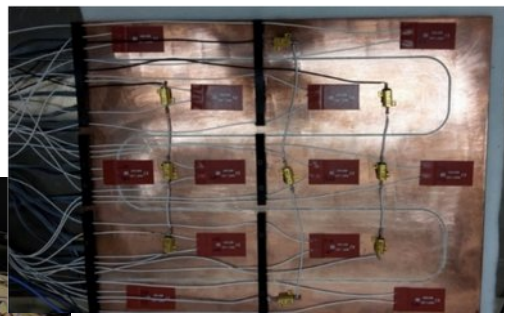
Active cooling test layout (400mm x 300mm x 3mm thick copper plate with 1,80D pipes embedded)
