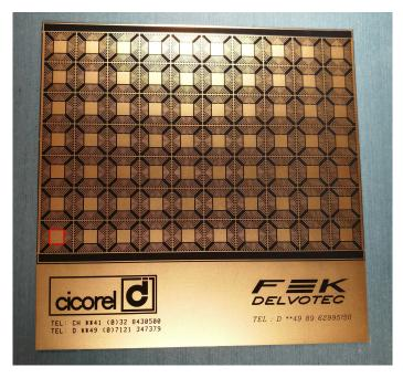
Figure 3.13: Photograph of the wire bond test material by *Cicorel*. The structure highlighted with red color indicates the regions used for test programs.
