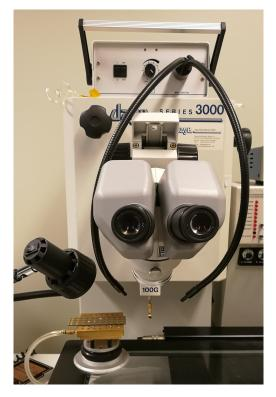
Figure 3.12: Photograph of the pull test machine *Dage Series 3000*. An extra light source is positioned on top of the pull test machine. The installed hook is a special hook which is only used for calibrations.
