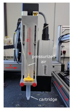
Figure 4.2: Photograph of the self made dispensing robot.
