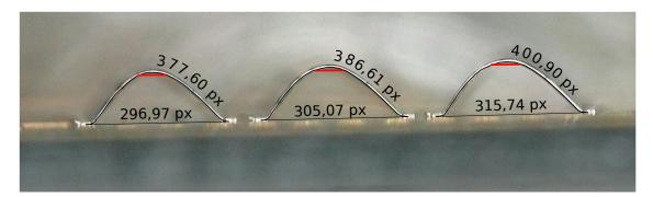
Figure 3.15: Microscope picture of the test program wire geometry. The red bar illustrates the estimated region of the position of the pull hook.
