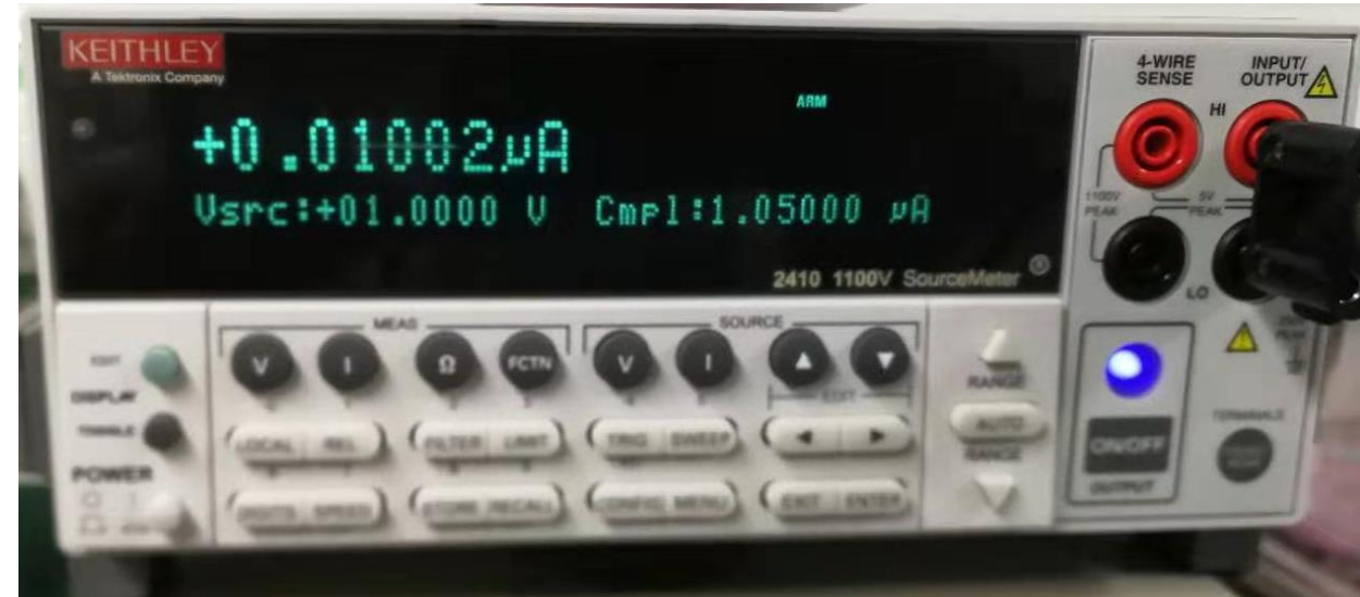
Fig : 1\text{V}/1\text{M}\Omega = 0.01\mu\text{A} with fluctuation
