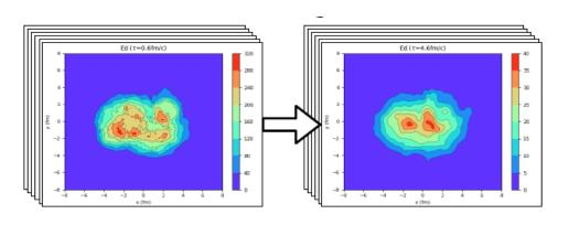
With the well trained network, the final state profiles can be quickly generated from the initial profiles. (5-10 times faster for GPU based calculations)
