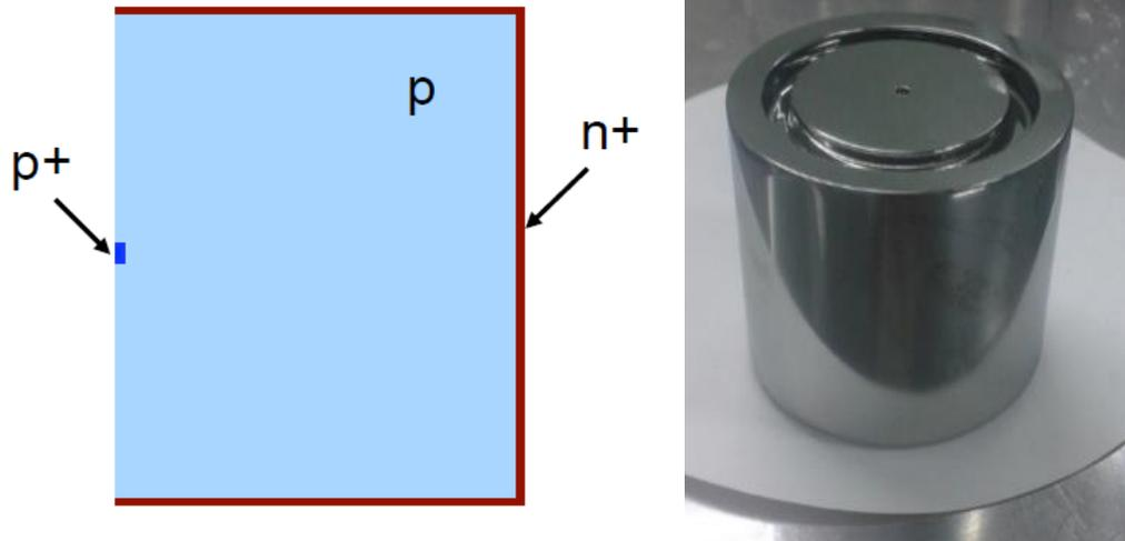
Direct detection of low-mass WIMPs w/ Ge detector at CJPL.
