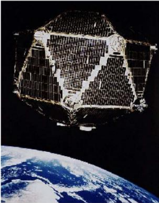
Sketch of one of the Vela satellites to search for violations of the nuclear test ban treaty.
