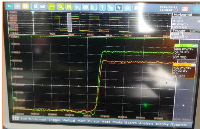
Synchronous clock signal test
