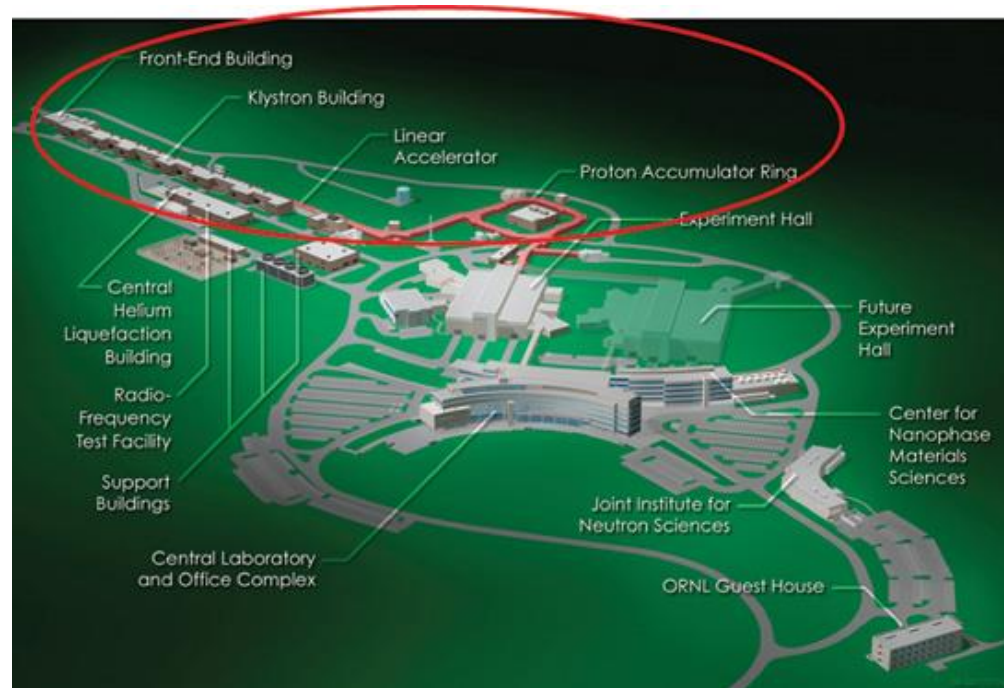
Figure 1: Oak Ridge National Laboratory's Spallation Neutron Source Uses a Linear Accelerator and Accumulator Ring to Generate a 1.4MW pulsed proton beam.
