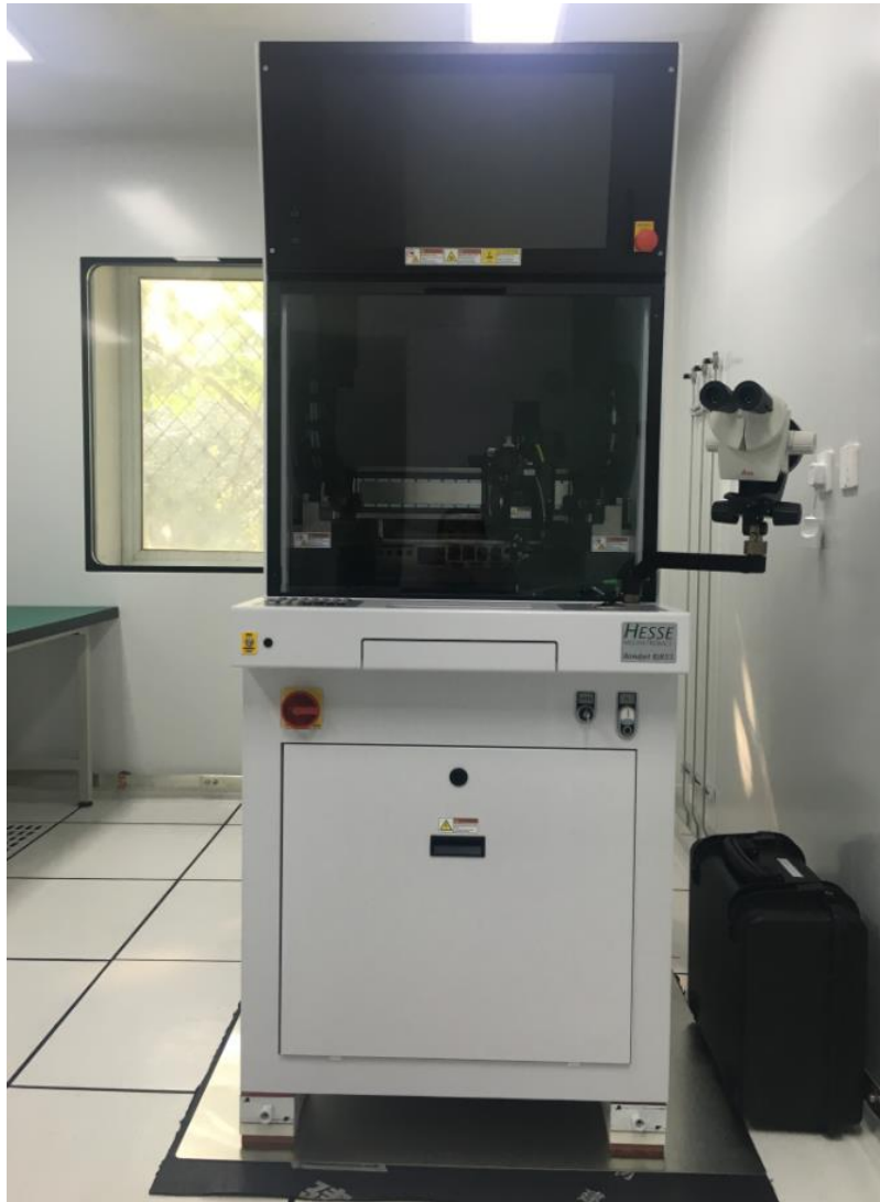
High Speed Fully Automatic Fine Wire Wedge Bonder @IHEP
