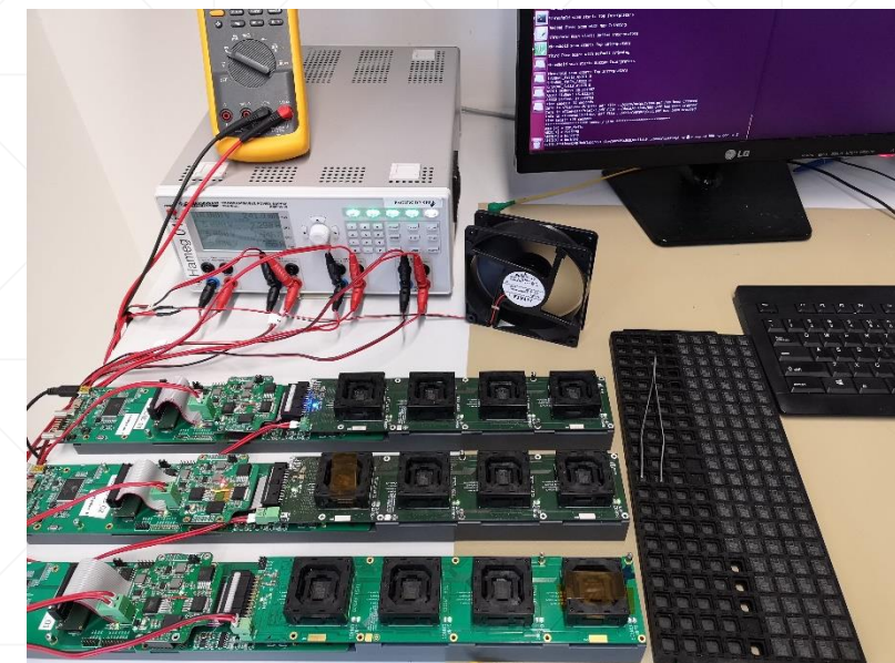
QA test running : 10 ASICs/run , ~100ASICs/hour
