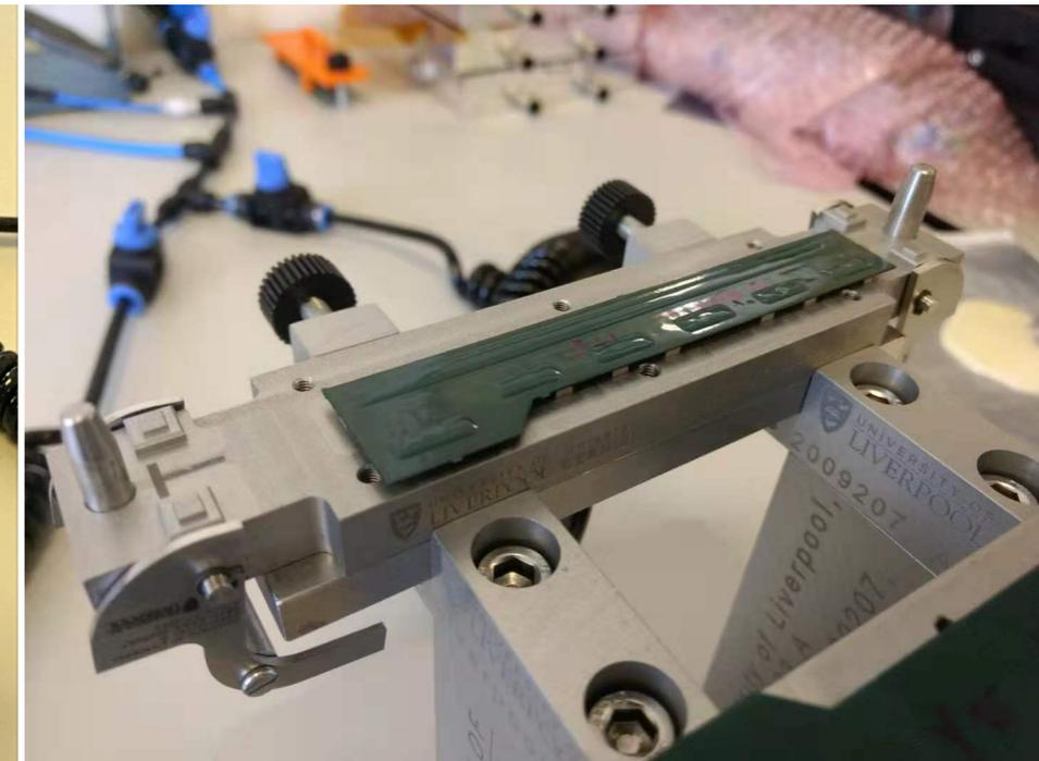
Hybrids are placed on sensor and left over night to cure
