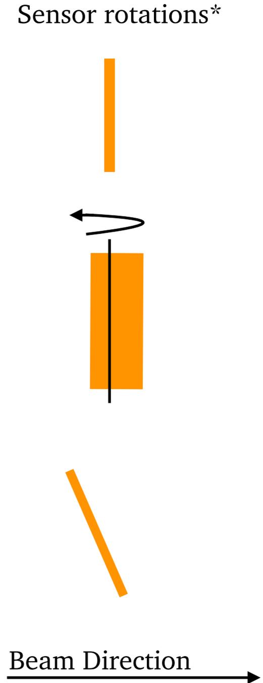
\* The sensors are mounted such that the strips are vertical
