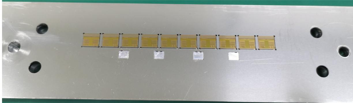
ASICs picked up using vacuum pick up tool
