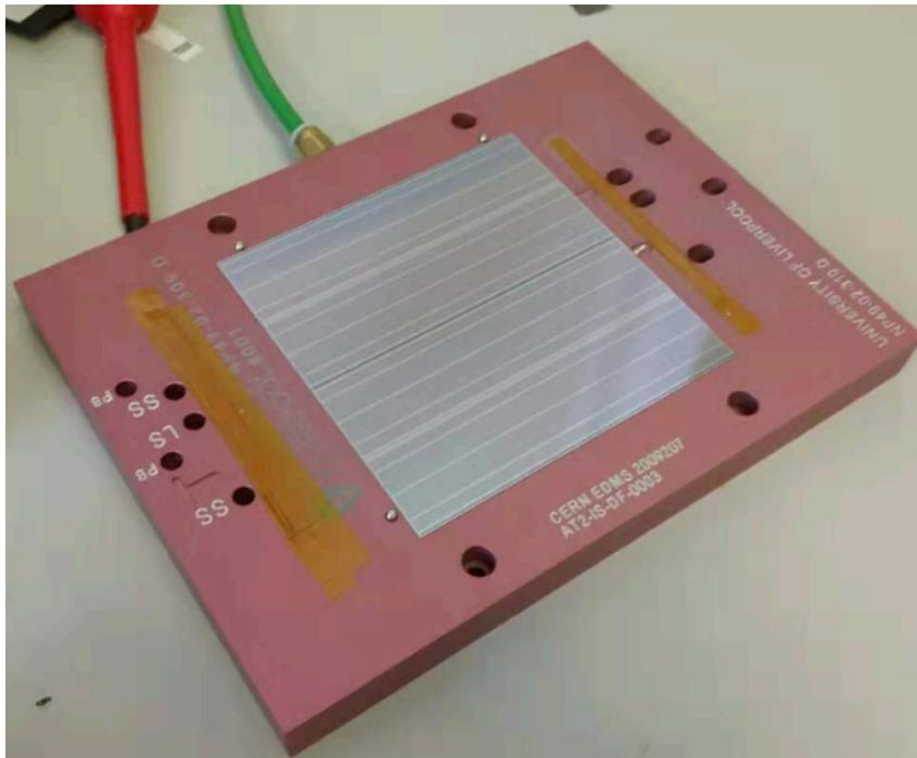
Stencil is then placed on top of the hybrids and glue is applied
