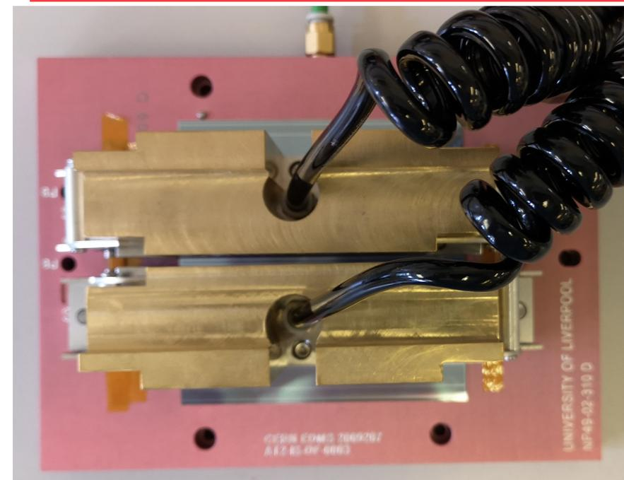
Sensor and hybrids after glue curing
