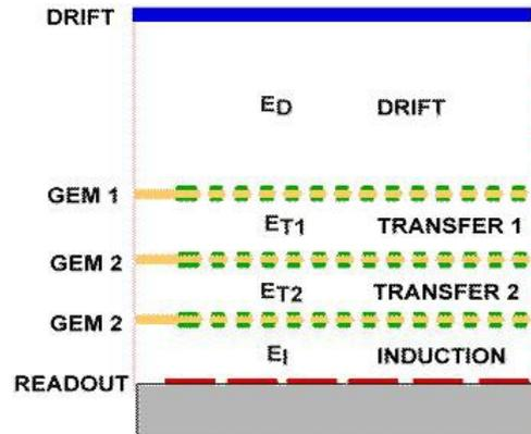
By stacking more foils together high gain can be reached with lower HV
