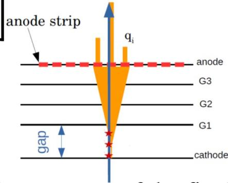
position reconstructed as average of the fired strip weighted by the charge on each strip
