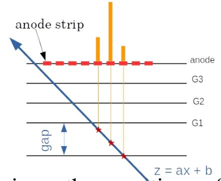
drift gap as a TPC gives the position of each ionization by the drift time and velocity  $\rightarrow$  linear fit
