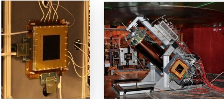
Testbeams to set the GEM working point
