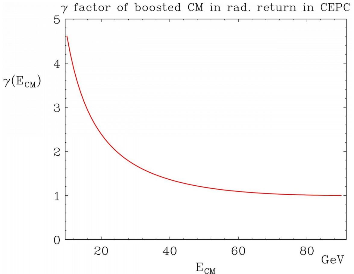
Derivation of the  $\gamma = E_{lab}/E_{CM}$  factor of the boosted  $e^+e^-$  system after  $e^+$  or  $e^-$  emits a hard photon.
