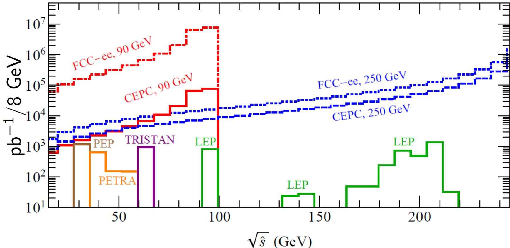
Integrated luminosity from past low energy  $e^+e^-$  colliders at their nominal center-of-mass energies compared to the effective luminosity through radiative return from future  $e^+e^-$  colliders at  $\sqrt{s} = 90$  or 250 GeV
