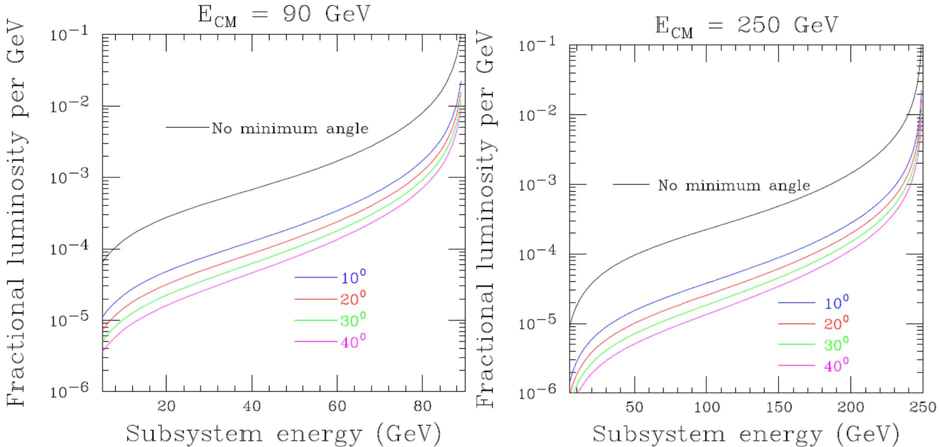
larger cut on photon angle  $\rightarrow$  cleaner signal, but less  $\sigma$
