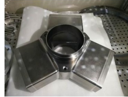
650 MHz 5-cell cavity with waveguide HOM coupler
