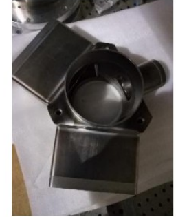
650 MHz 5-cell cavity with waveguide HOM coupler
